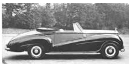
Here is SHD50 as it was delivered to Jean Simon in May 1953. The unique body design 7296 distinctly shows the Jensen rear type window, the low line of the folded hood and the two light design of the side made for the shortened body.
