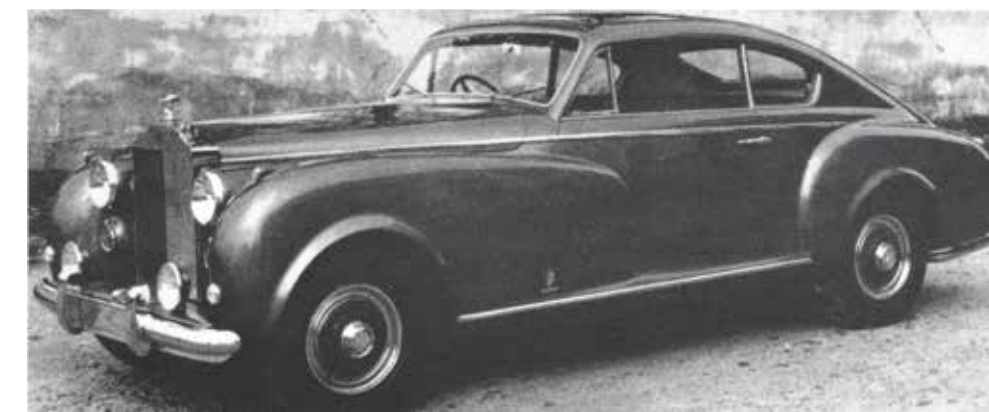
The one-off body by famous French coachbuilder Chapron on chassis LSTH79 shows a similar 2-light hood design. However this design by Chapron was executed long after H.J. Mulliner's design on SHD50.
